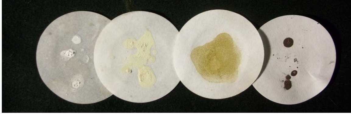
Figure 14. The microcrystalline powder obtained from crystal growth in 2.5” silver ampoules. This crystal growth focuses on the feasibility of alloying \text{ThO}_2 with U. From left to right the reactions were set up to produce \text{ThO}_2 , \text{U}_{0.1}\text{Th}_{0.9}\text{O}_2 , \text{U}_{0.5}\text{Th}_{0.5}\text{O}_2 , and \text{UO}_2 . However, using EDX, no uranium was found in the \text{U}_{0.1}\text{Th}_{0.9}\text{O}_2 reaction. Additionally, the \text{U}_{0.5}\text{Th}_{0.5}\text{O}_2 was measured to contain roughly 33% uranium, while the \text{UO}_2 is simply a \text{UO}_x compound. X-ray diffraction needs to be done to confirm the identity of the \text{UO}_x species.
