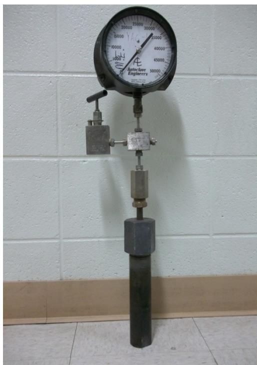
Figure 10. An assembled Tuttle cold-cone seal autoclave used in this study. The autoclave consists of an Inconel 718 chamber and cap nut, high pressure tubing, pressure relief valve, and pressure gauge. The pressure relief valve is used to vent reactions that have been overfilled, either intentionally or unintentionally.
