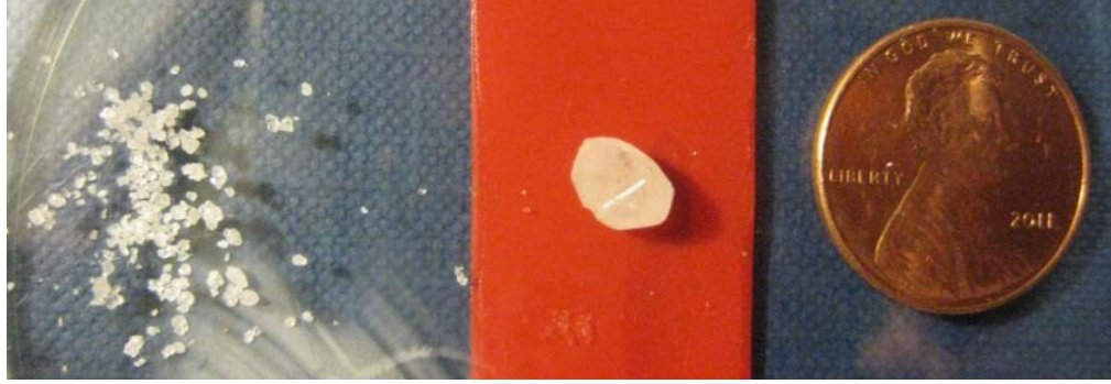
Figure 13. Comparison of nucleation produced during \text{ThO}_2 bulk growth using 12M CsF and a gradient of 670-635°C. The nucleation appeared to have come directly from the solution. Nucleation along the walls of the ampoules is often thin, rounded plates with small clusters of crystals. Characteristics of the reaction products guided future crystal synthesis experiments.
