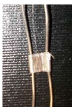
Figure 8. A crystal ladder made from 1mm silver wire using 1/4" silver tubing as rungs. The seed crystal is suspended from 0.1mm silver wire that has been tied between two rungs. Using several seeds on a single ladder can be a way to explore synthesis at different temperatures.
